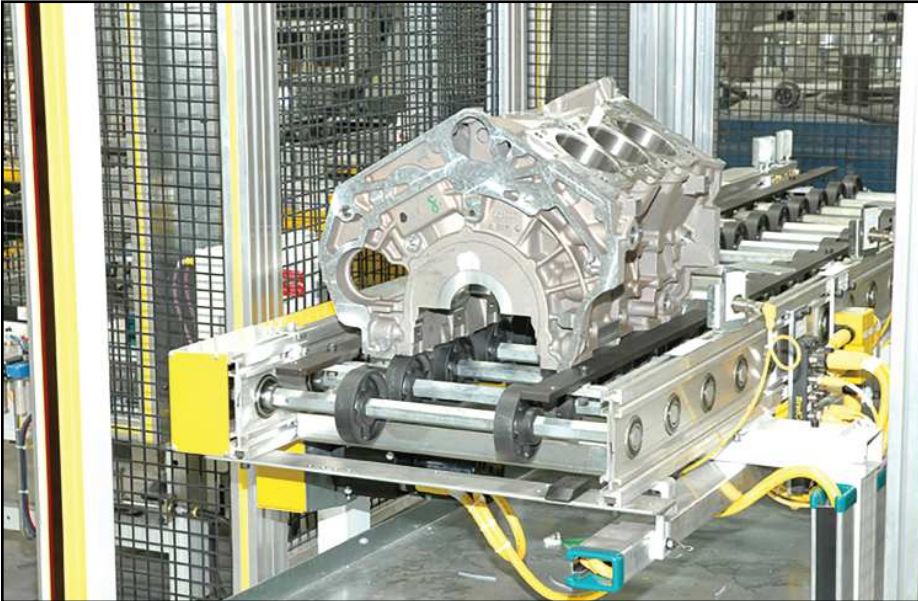
Reversing Inspection Stations
